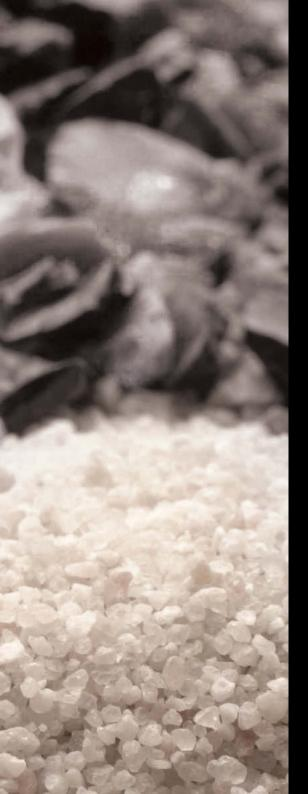
TechniStone<sup>®</sup> is made from natural materials (quartz and granite) and a high-quality binding agent, supplemented with coloured pigments and glass or mirror granules. In the form of highly durable large-size boards, hardened stone is widely used in the private, public and industrial sectors.
